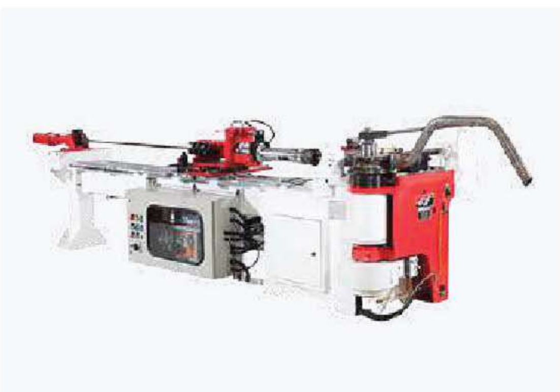
Hydraulic NC Pipe Bending
